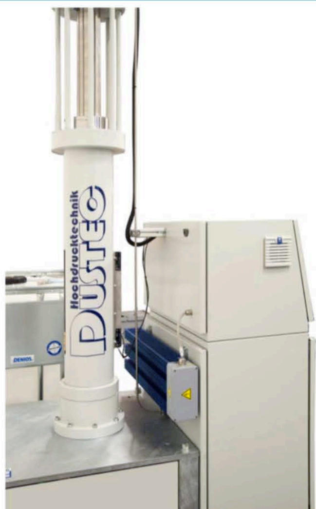
Figure 6: Electromechanical Pressure Generator (EPG) 7 000 bar, with Control Unit (PLC, Touch-panel), pre- pressure pump
